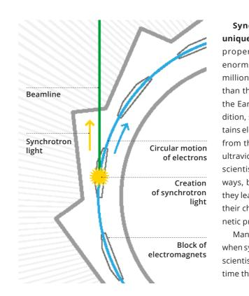
million laps in one second! In order for the electrons to rush around on a closed-loop path, their movement path is curved by twelve blocks of electromagnets. Electromagnetic radiation called synchrotron light is generated in the places where the path of the electrons is curved.
