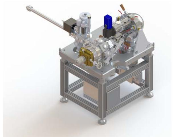
Figure 7: Photoemission Electron Microscope (PEEM) meant for the Solaris.
