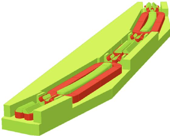
Figure 5: Magnet half block with coils in red [9].
