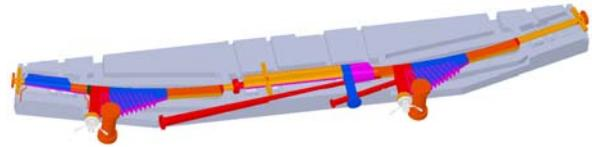
Figure 6: View of the DBA magnet (lower half) with the vacuum chamber inserted [11].
