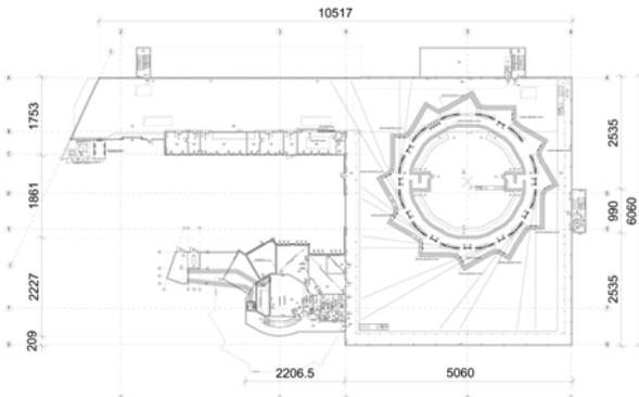
Figure 4: Concept of the facility layout on level  $-3.2$  m. The experimental hall can be extended by about  $10 \text{ m}$  on the right hand side in the future. Above the linac tunnel ample covered space is available for pre-assembly and general laboratories. Dimensions in centimetres.
