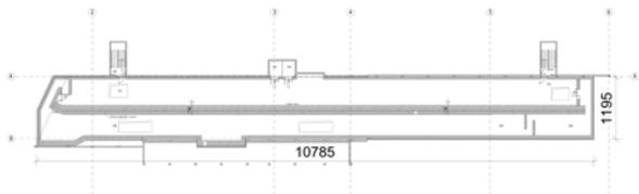
Figure 3: Concept of the modulator and service gallery (above) and linac tunnel (below) layout on level  $-7.7$  m. Dimensions in centimetres.
