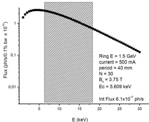
Figure 8: Theoretical synchrotron radiation flux profile from superconducting 3.75 T wiggler. Rectangle indicate possible to use energy range [15].
