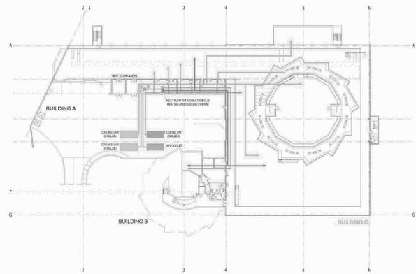
Figure 3: Schematics of the water cooling system.
