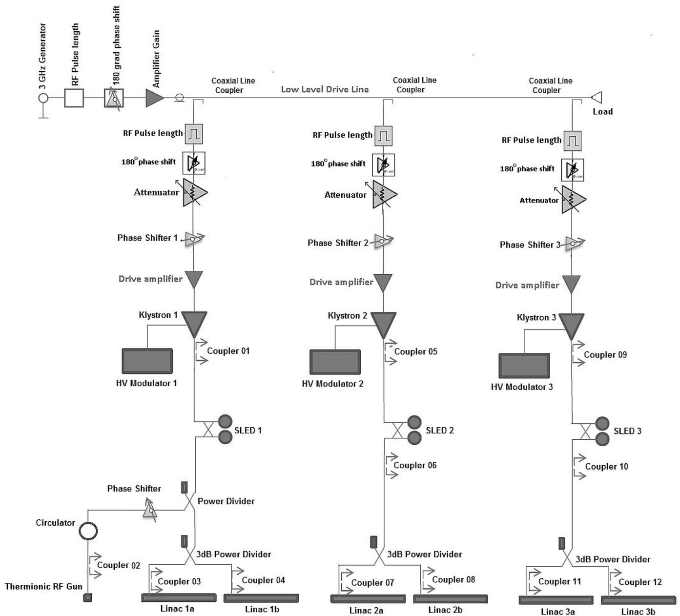
Figure 3. Diagram of the RF system for SOLARIS injector
