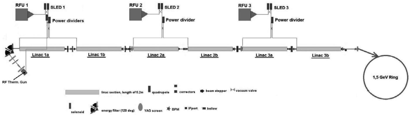
Figure 1. Layout of SOLARIS injector
