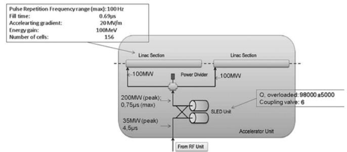
Figure 2. Schematic layout of accelerator unit
